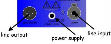
Typical connection set-up for the PHILTER
